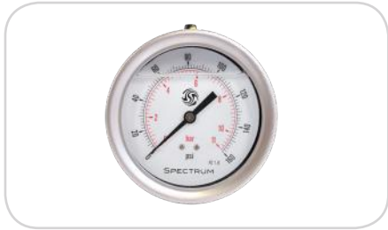
SPECTRUM Gauges (PG3) 11 bar ¼" glycerine filled stainless steel back mounted pressure gauge.
