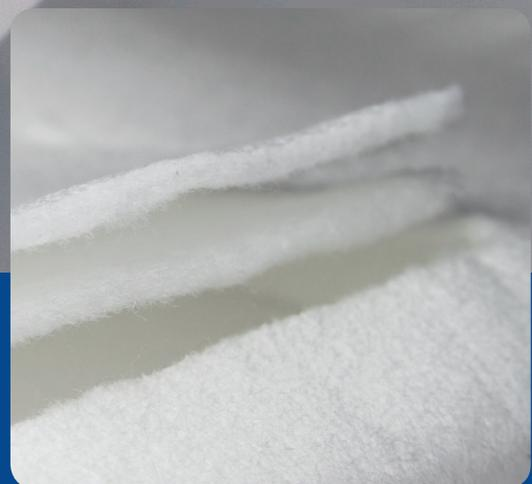
“pre-filter” layer traps larger particles and gelatinous contaminants, which often cause premature blinding, with the second, finer filtration layer effectively trapping unwanted particulate.
